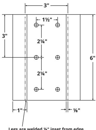
Legs are welded 1/8" inset from edge of leg bracket.
