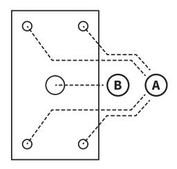
\*Screw "B" must be installed to ensure additional top cap strength. \*Vitro Seating Products can not guarantee installation compatibility on existing booths.
